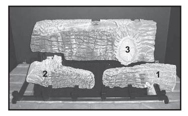
**STEP 4:** (SRV2057-722): Place log 3 so that the bottom notches mate with the 2 back steel tabs. Tab A is located on the right side of pilot bracket, tab B is located at the back/right corner of burner. NOTE: There should be a 1/2 inch gap between the bottom of log 3 and the top edge of the burner. The underside of log #3 must not cover ANY burner ports.
